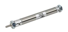
NITRA pneumatic cylinder, non-repairable, 9/16in bore, 3/16in rod diameter, 3in stroke, double acting, magnetic piston, double end mount.
