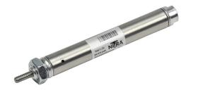
NITRA pneumatic cylinder, non-repairable, 9/16in bore, 3/16in rod diameter, 2in stroke, single acting, front nose mount.
