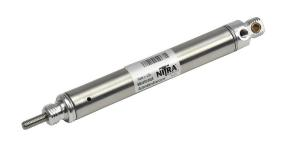
NITRA pneumatic cylinder, non-repairable, 9/16in bore, 3/16in rod diameter, 2in stroke, single acting, double end mount.
