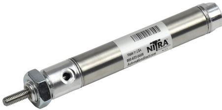
NITRA pneumatic cylinder, non-repairable, 9/16in bore, 3/16in rod diameter, 2in stroke, double acting, front nose mount.
