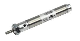
NITRA pneumatic cylinder, non-repairable, 9/16in bore, 3/16in rod diameter, 2in stroke, double acting, front nose mount.
