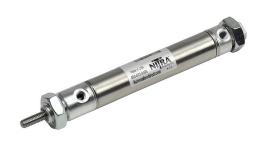
NITRA pneumatic cylinder, non-repairable, 9/16in bore, 3/16in rod diameter, 2in stroke, double acting, double end mount.
