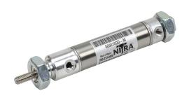
NITRA pneumatic cylinder, non-repairable, 9/16in bore, 3/16in rod diameter, 1in stroke, double acting, magnetic piston, double end mount.
