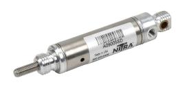
NITRA pneumatic cylinder, non-repairable, 9/16in bore, 3/16in rod diameter, 1/2in stroke, single acting, double end mount.
