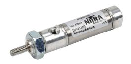
NITRA pneumatic cylinder, non-repairable, 9/16in bore, 3/16in rod diameter, 1/2in stroke, double acting, front nose mount.
