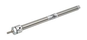
NITRA pneumatic cylinder, non-repairable, 7/16in bore, 3/16in rod diameter, 6in stroke, double acting, front nose mount.
