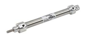
NITRA pneumatic cylinder, non-repairable, 7/16in bore, 3/16in rod diameter, 3in stroke, double acting, rear pivot mount.
