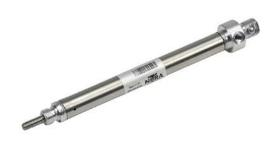
NITRA pneumatic cylinder, non-repairable, 7/16in bore, 3/16in rod diameter, 2in stroke, single acting, rear pivot mount.
