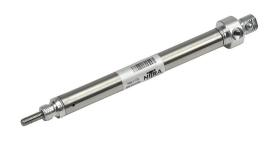
NITRA pneumatic cylinder, non-repairable, 7/16in bore, 3/16in rod diameter, 2in stroke, single acting, rear pivot mount.
