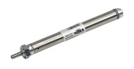
NITRA pneumatic cylinder, non-repairable, 7/16in bore, 3/16in rod diameter, 2in stroke, single acting, front nose mount.
