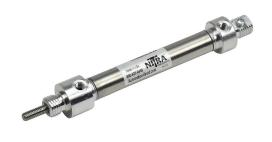
NITRA pneumatic cylinder, non-repairable, 7/16in bore, 3/16in rod diameter, 2in stroke, double acting, rear pivot mount.
