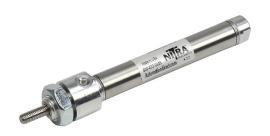
NITRA pneumatic cylinder, non-repairable, 7/16in bore, 3/16in rod diameter, 2in stroke, double acting, front nose mount.
