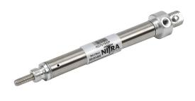
NITRA pneumatic cylinder, non-repairable, 7/16in bore, 3/16in rod diameter, 1-1/2in stroke, single acting, rear pivot mount.
