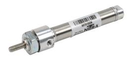
NITRA pneumatic cylinder, non-repairable, 7/16in bore, 3/16in rod diameter, 1-1/2in stroke, double acting, front nose mount.
