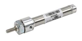
NITRA pneumatic cylinder, non-repairable, 7/16in bore, 3/16in rod diameter, 1 1/2in stroke, double acting, front nose mount.
