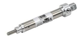
NITRA pneumatic cylinder, non-repairable, 7/16in bore, 3/16in rod diameter, 1in stroke, single acting, rear pivot mount.
