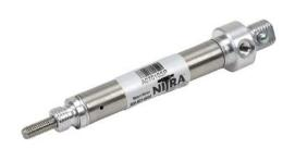
NITRA pneumatic cylinder, non-repairable, 7/16in bore, 3/16in rod diameter, 1in stroke, single acting, rear pivot mount.
