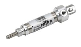
NITRA pneumatic cylinder, non-repairable, 7/16in bore, 3/16in rod diameter, 1/2in stroke, single acting, rear pivot mount.
