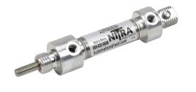
NITRA pneumatic cylinder, non-repairable, 7/16in bore, 3/16in rod diameter, 1/2in stroke, double acting, rear pivot mount.
