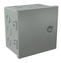
Wiegmann enclosure, NEMA 1, 6 x 6 x 4in (HxWxD), wall mount, with knockouts, carbon steel, ANSI 61 gray, powder coat finish, single-door, integral snap-tight latch.
