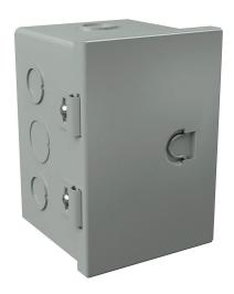
Wiegmann enclosure, NEMA 1, 6 x 4 x 4in (HxWxD), wall mount, with knockouts, carbon steel, ANSI 61 gray, powder coat finish, single-door, integral snap-tight latch.
