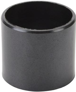
igus iglide series plain bearing, type T500 polymer, 1in inside diameter, 1-1/8in outside diameter, 1in overall length. Package of 2. For use with 1in diameter drylin R series shafts.
