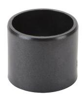
igus iglide series plain bearing, type T500 polymer, 3/4in inside diameter, 7/8in outside diameter, 3/4in overall length. Package of 2. For use with 3/4in diameter drylin R series shafts.
