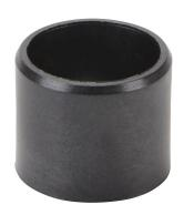
igus iglide series plain bearing, type T500 polymer, 1/2in inside diameter, 9/16in outside diameter, 1/2in overall length. Package of 5. For use with 1/2in diameter drylin R series shafts.
