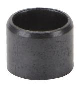
igus iglide series plain bearing, type T500 polymer, 1/4in inside diameter, 5/16in outside diameter, 1/4in overall length. Package of 5. For use with 1/4in diameter drylin R series shafts.
