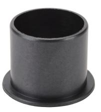
igus iglide series plain bearing, type T500 polymer, 1in inside diameter, 1-1/8in outside diameter, 1in overall length, flanged. Package of 2. For use with 1in diameter drylin R series shafts.
