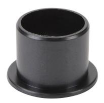
igus iglide series plain bearing, type T500 polymer, 3/4in inside diameter, 7/8in outside diameter, 3/4in overall length, flanged. Package of 2. For use with 3/4in diameter drylin R series shafts.
