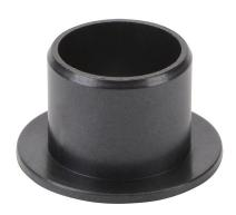
igus iglide series plain bearing, type T500 polymer, 1/2in inside diameter, 9/16in outside diameter, 1/2in overall length, flanged. Package of 5. For use with 1/2in diameter drylin R series shafts.
