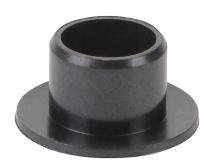
igus iglide series plain bearing, type T500 polymer, 1/4in inside diameter, 5/16in outside diameter, 1/4in overall length, flanged. Package of 5. For use with 1/4in diameter drylin R series shafts.
