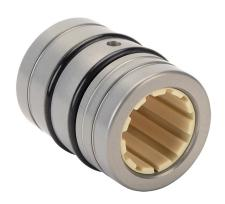
igus drylin R series plain bearing, type J polymer bearing, 3/4in inside diameter, 1-5/8in overall length, self-aligning housing, closed, anodized aluminum.
