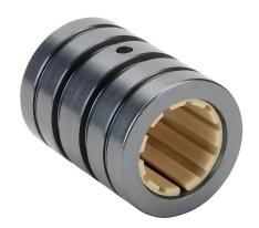
igus drylin R series plain bearing, type J polymer bearing, 3/4in inside diameter, 1-5/8in overall length, fixed housing, closed, anodized aluminum.
