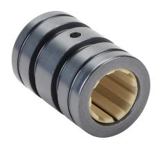
igus drylin R series plain bearing, type J polymer bearing, 1/2in inside diameter, 1-1/4in overall length, fixed housing, closed, anodized aluminum.
