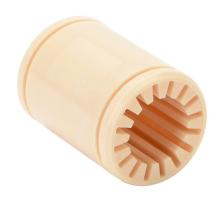
igus drylin R series plain bearing, type J polymer bearing, 1/2in inside diameter, 1-1/4in overall length, fixed housing, closed, type J polymer.
