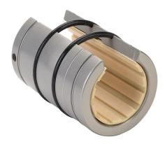
igus drylin R series plain bearing, type J polymer bearing, 1in inside diameter, 2-1/4in overall length, self-aligning housing, open, anodized aluminum.
