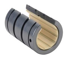
igus drylin R series plain bearing, type J polymer bearing, 1in inside diameter, 2-1/4in overall length, fixed housing, open, anodized aluminum.
