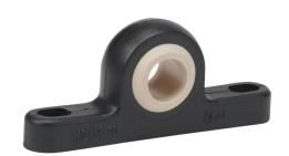
igus igubal K series mounted spherical bearing, type L280 polymer bearing, 10mm inside diameter, pillow block, igumid G polymer. For use with drylin R series 10mm shafts.
