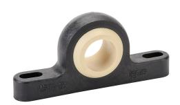
igus igubal K series mounted spherical bearing, type L280 polymer bearing, 3/4in inside diameter, pillow block, igumid G polymer.
