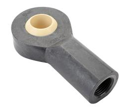
igus igubal K series mounted spherical bearing, type L280 polymer bearing, 1in inside diameter, 1.375in width, 1-12 UNF female thread rod end, igumid G polymer.
