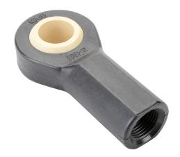
igus igubal K series mounted spherical bearing, type L280 polymer bearing, 3/4in inside diameter, 0.875in width, 3/4-16 UNF female thread rod end, igumid G polymer.
