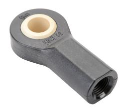
igus igubal K series mounted spherical bearing, type L280 polymer bearing, 1/2in inside diameter, 0.625in width, 1/2-20 UNF female thread rod end, igumid G polymer. Package of 2
