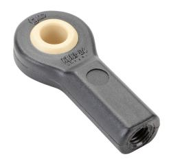
igus igubal K series mounted spherical bearing, type L280 polymer bearing, 1/4in inside diameter, 0.365in width, 1/4-28 UNF female thread rod end, igumid G polymer. Package of 4.
