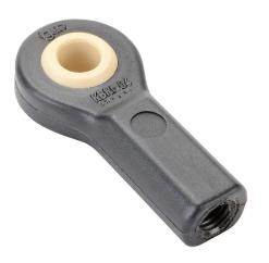
igus igubal K series mounted spherical bearing, type L280 polymer bearing, 1/4in inside diameter, 0.365in width, 1/4-28 UNF female thread rod end, igumid G polymer. Package of 4.
