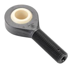
igus igubal K series mounted spherical bearing, type L280 polymer bearing, 1/2in inside diameter, 0.625in width, 1/2-20 UNF male thread rod end, igumid G polymer. Package of 2.
