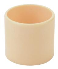
igus iglide series plain bearing, type J polymer, 1in inside diameter, 1-1/8in outside diameter, 1in overall length. Package of 2. For use with 1in diameter drylin R series shafts.
