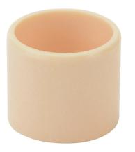
igus iglide series plain bearing, type J polymer, 3/4in inside diameter, 7/8in outside diameter, 3/4in overall length. Package of 5. For use with 3/4in diameter drylin R series shafts.
