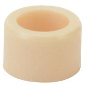
igus iglide series plain bearing, type J polymer, 1/4in inside diameter, 3/8in outside diameter, 1/4in overall length. Package of 10. For use with 1/4in diameter drylin R series shafts.
