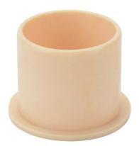
igus iglide series plain bearing, type J polymer, 1in inside diameter, 1-1/8in outside diameter, 1in overall length, flanged. Package of 2. For use with 1in diameter drylin R series shafts.
