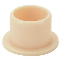
igus iglide series plain bearing, type J polymer, 1/2in inside diameter, 5/8in outside diameter, 1/2in overall length, flanged. Package of 10. For use with 1/2in diameter drylin R series shafts.
