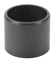
igus iglide series plain bearing, type G300 polymer, 3/4in inside diameter, 7/8in outside diameter, 3/4in overall length. Package of 5. For use with 3/4in diameter drylin R series shafts.
