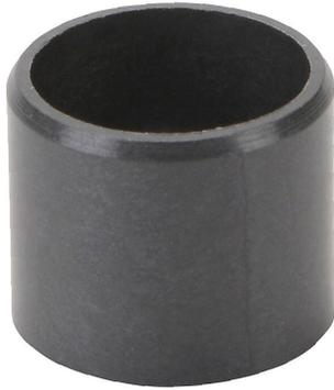
igus iglide series plain bearing, type G300 polymer, 1/2in inside diameter, 9/16in outside diameter, 1/2in overall length. Package of 10. For use with 1/2in diameter drylin R series shafts.
