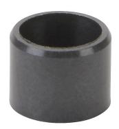
igus iglide series plain bearing, type G300 polymer, 1/4in inside diameter, 5/16in outside diameter, 1/4in overall length. Package of 10. For use with 1/4in diameter drylin R series shafts.
